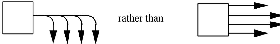
3. Control feedbacks shall be shown as "up and over."
