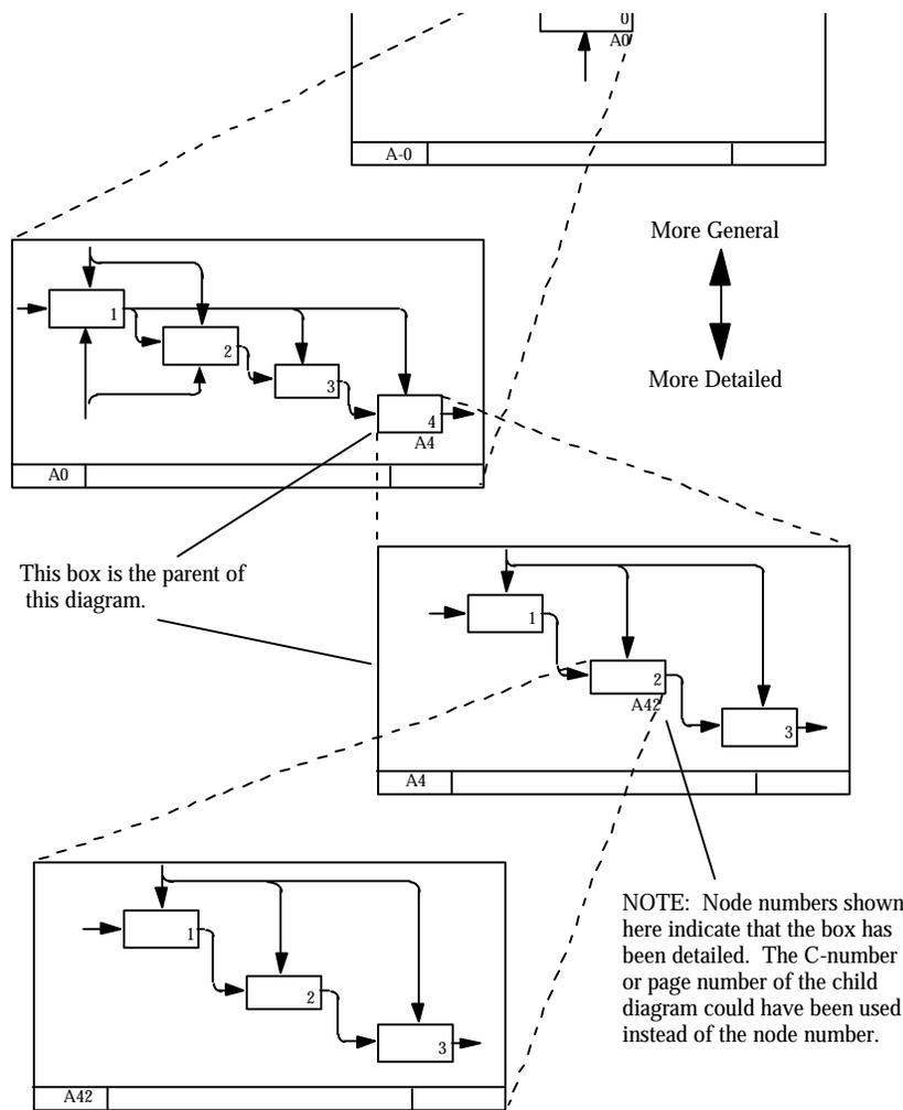
The single function represented on the top-level context diagram may be decomposed into its major sub-functions by creating its child diagram. In turn, each of these sub-functions may be decomposed, each creating another, lower-level child diagram. On a given diagram, some of the functions, none of the functions or all of the functions may be decomposed. Each child diagram contains the child boxes and arrows that provide additional detail about the parent box.
