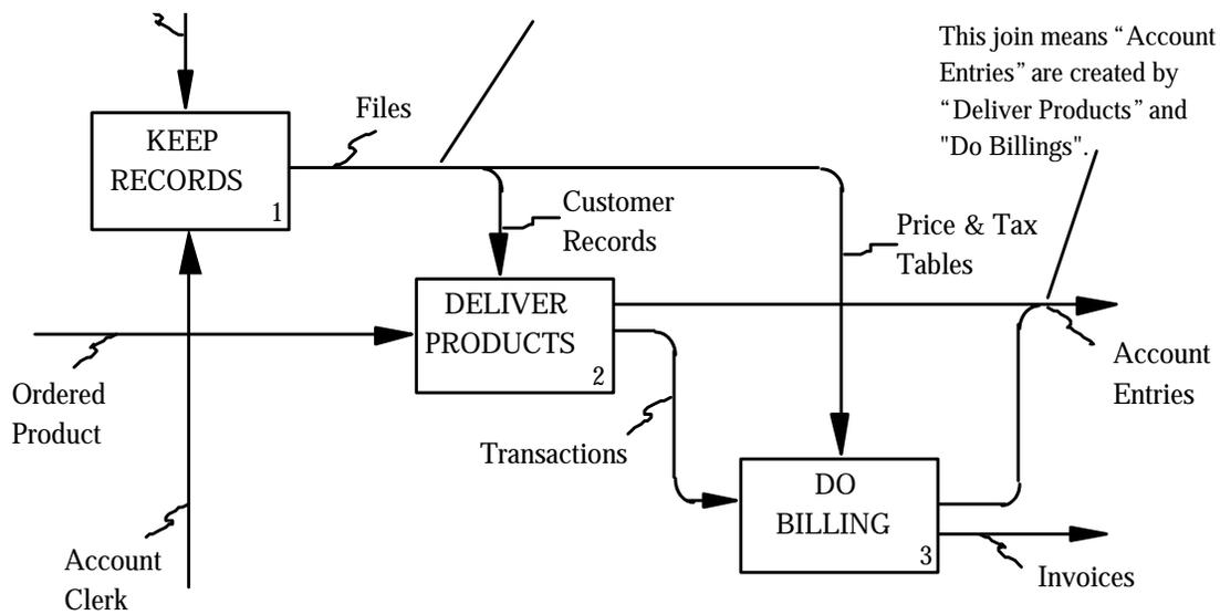
**Figure 12. Connections Between Boxes**
