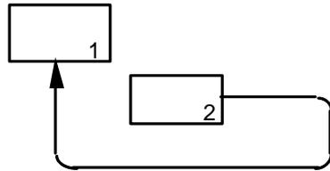
13. The unconnected end of a boundary arrow shall have the proper ICOM code specifying its connection to the parent box, or shall be tunneled.
