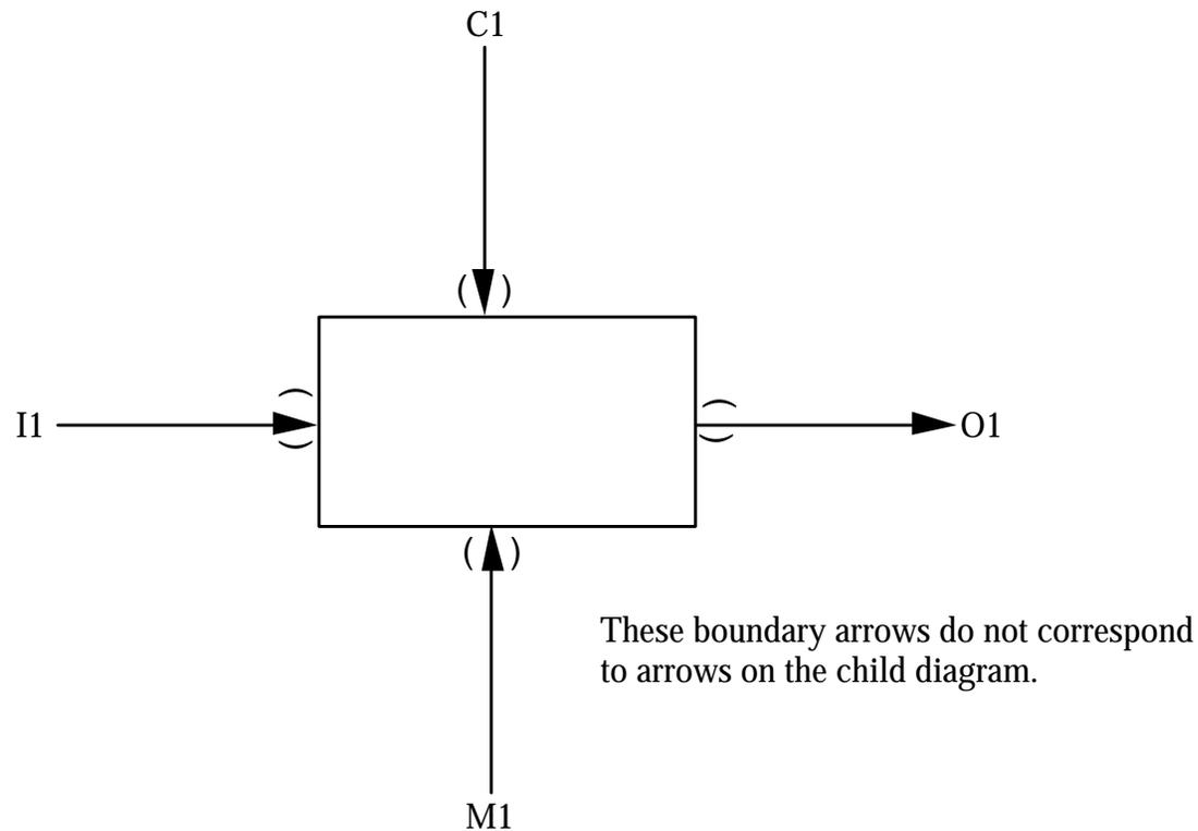
**Figure 16. Arrows Tunneled at Connected End**
