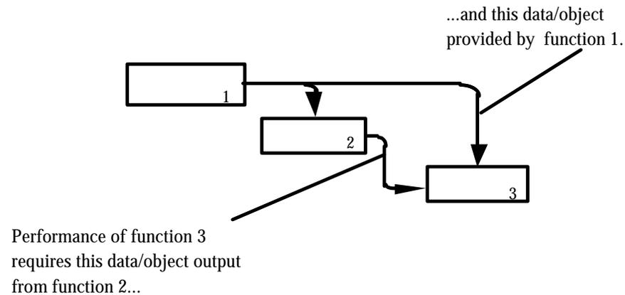
Figure 8. Meaning of Constraint
