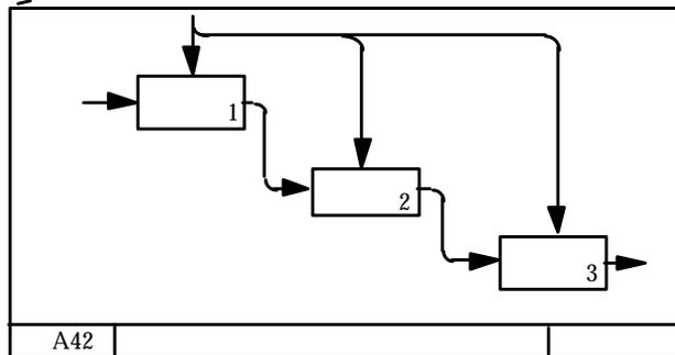
NOTE: Node numbers shown here indicate that the box has been detailed. The C-number or page number of the child diagram could have been used instead of the node number.
