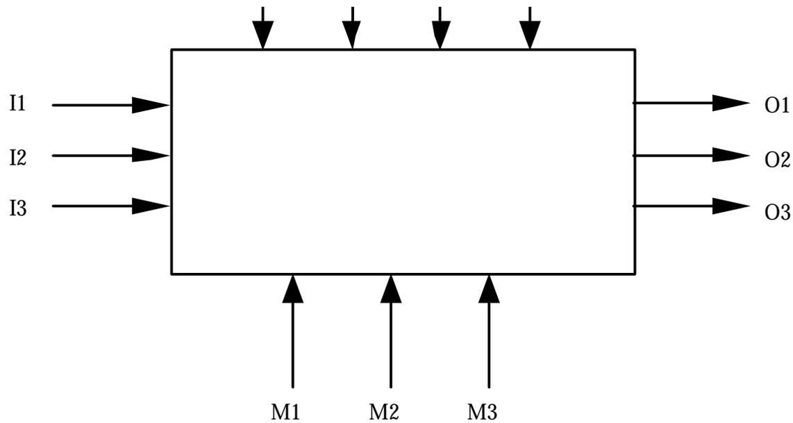
**Figure B8. Illustration of ICOM coding**
