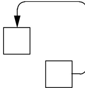
Input feedbacks shall be shown as "down and under."
