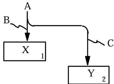
Pipeline A splits into B and C to provide controls to X and Y.
