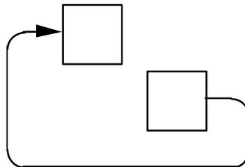
Mechanism feedback shall be shown as "down and under."
