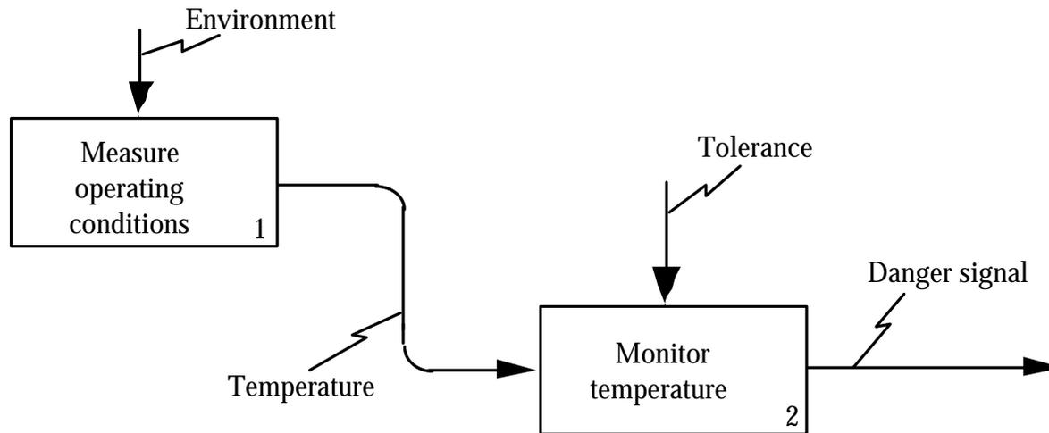
**Figure B6. Example of Constraint**
