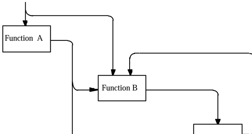
In Figure A2, Function B is constrained by one input and two controls, and produces a single output, which constrains Function C.
