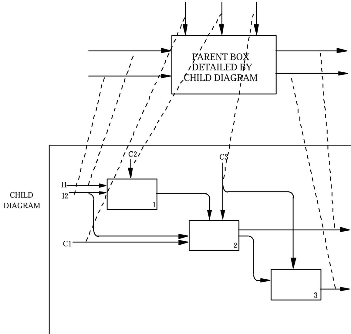
NOTE: The dashed lines show how the ICOMs on the child diagram relate boundary arrows on the child to the arrows of its parent box.
